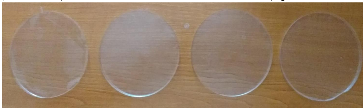
Figure 1 – HPMC/GONE multicomponent films with different GONE concentrations (0%, 2.5%, 5%, 7.5% GONE respectively)
