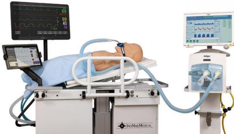
A virtual respiratory therapy simulator setup. It includes a mannequin lying on a gurney, connected to a ventilator. A monitor on the left displays vital signs: 69, 99, 40, and 14. A tablet is also visible. The ventilator on the right has a screen showing a waveform. The brand name 'INGMAR MEDICAL' is visible on the gurney. |
